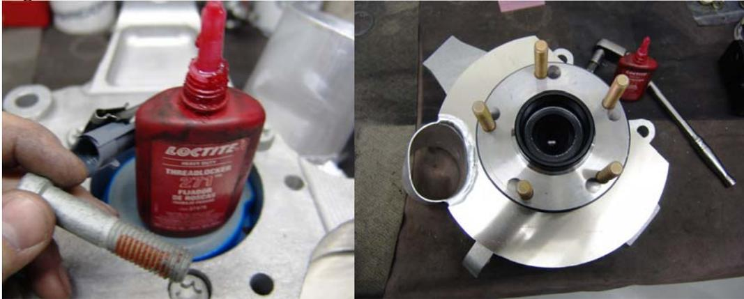
Before installing the bolts holding the assembly together you should apply a small amount of red loctite to the bolts and torque to manufacturer specification of 96 ft-lbs. At this time you should re-assemble the suspension as it was removed from the car.
